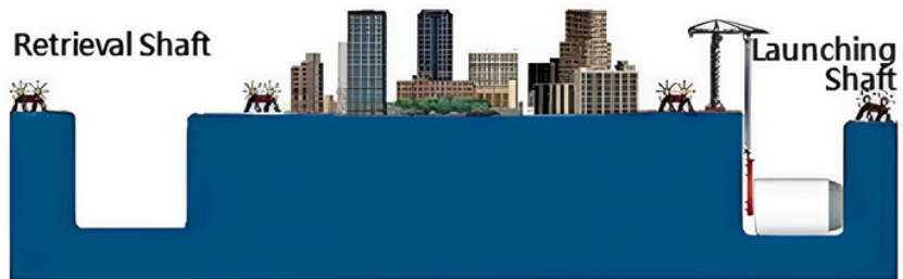
2. Assemble the TBM at the launching shaft
