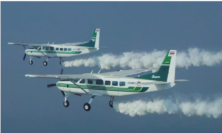
*Planes drop the chemicals to seed clouds during an artificial rain-making operation.*
