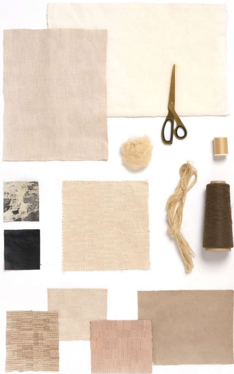
Pineapple leaf long and shot fiberW / Pineapple leaf fiber fabric / PU coating on pineapple leaf fiber fabric / Thread / Scissor
