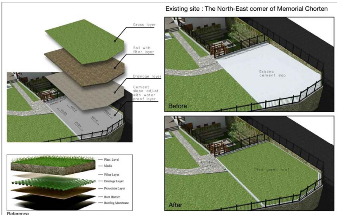
Figure Q5-37. Presentation of existing cement slab renovation at Memorial Chorten.
