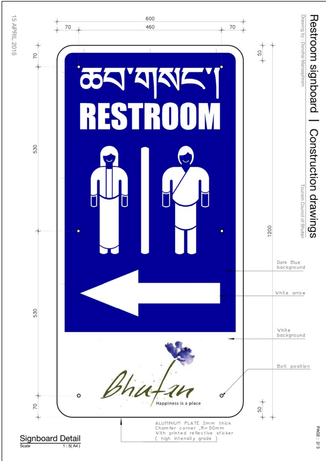
Figure Q1-11. Restrooms signboard final production drawings
