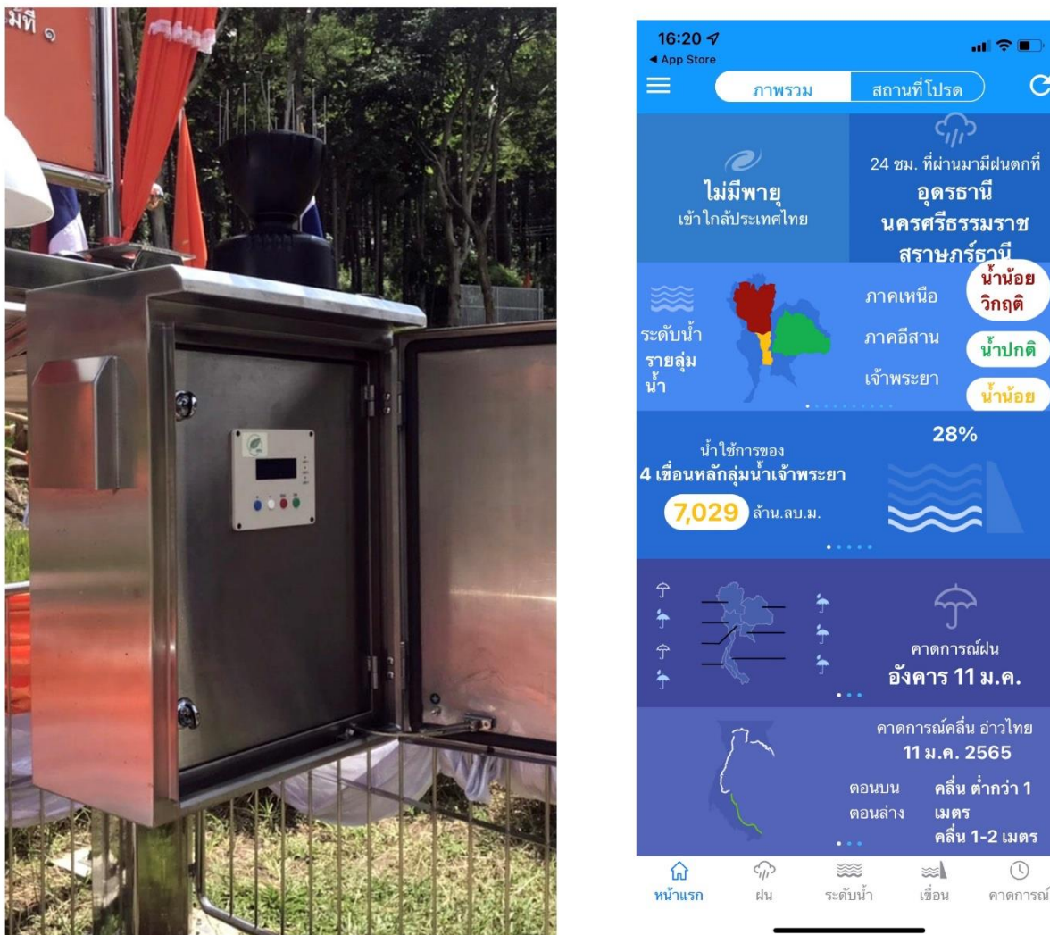
Photo: (from left to right) Automated Telemetry Station in Pongyeang sub-district, Mae Rim District, Chiang Mai Province and interface of ThaiWater mobile-application that has been integrated for general use.
