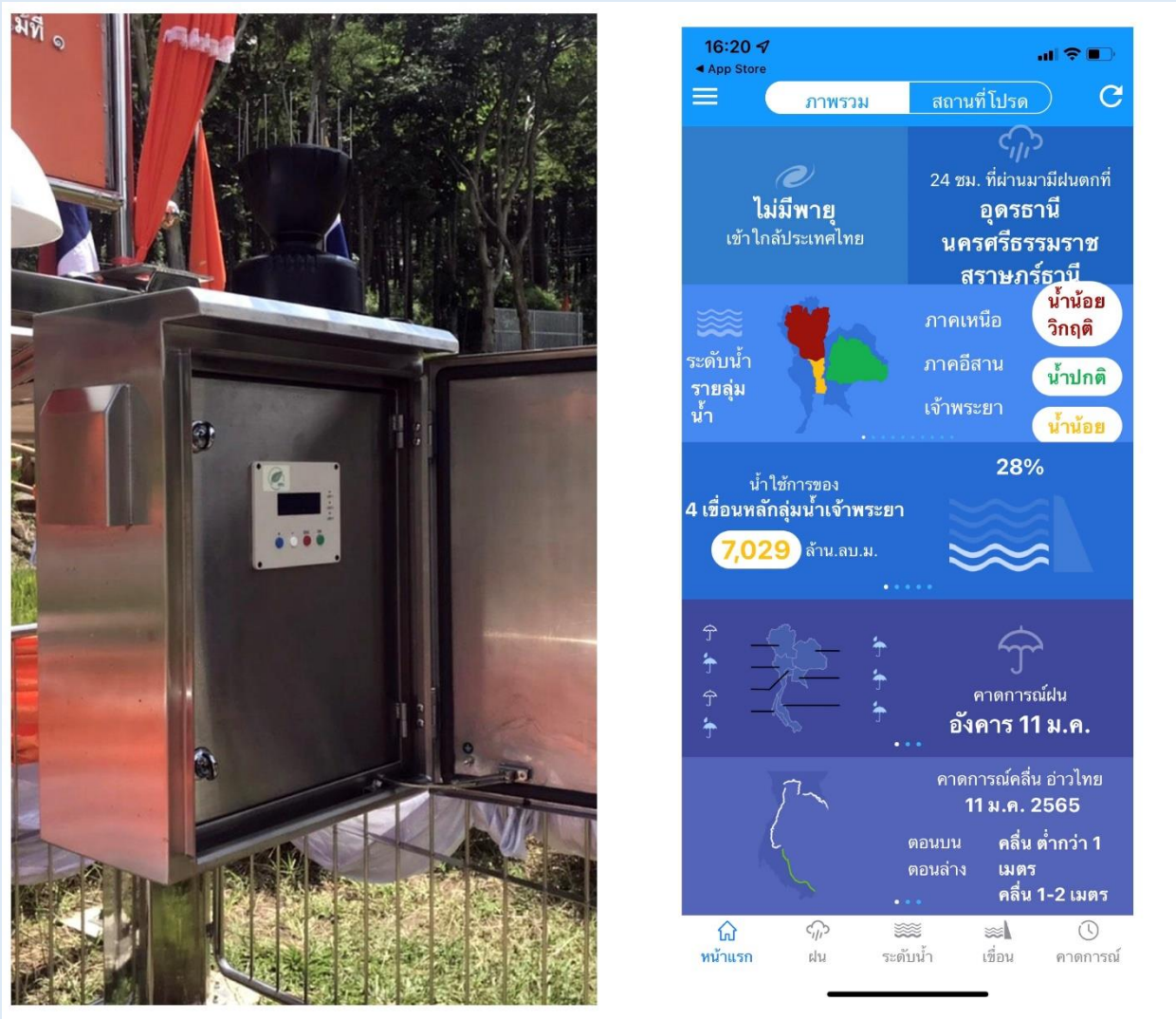
Photo: (from left to right) Automated Telemetry Station in Pongyeang sub-district, Mae Rim District, Chiang Mai Province and interface of ThaiWater mobile-application that has been integrated for general use. (Source: Matichon)
